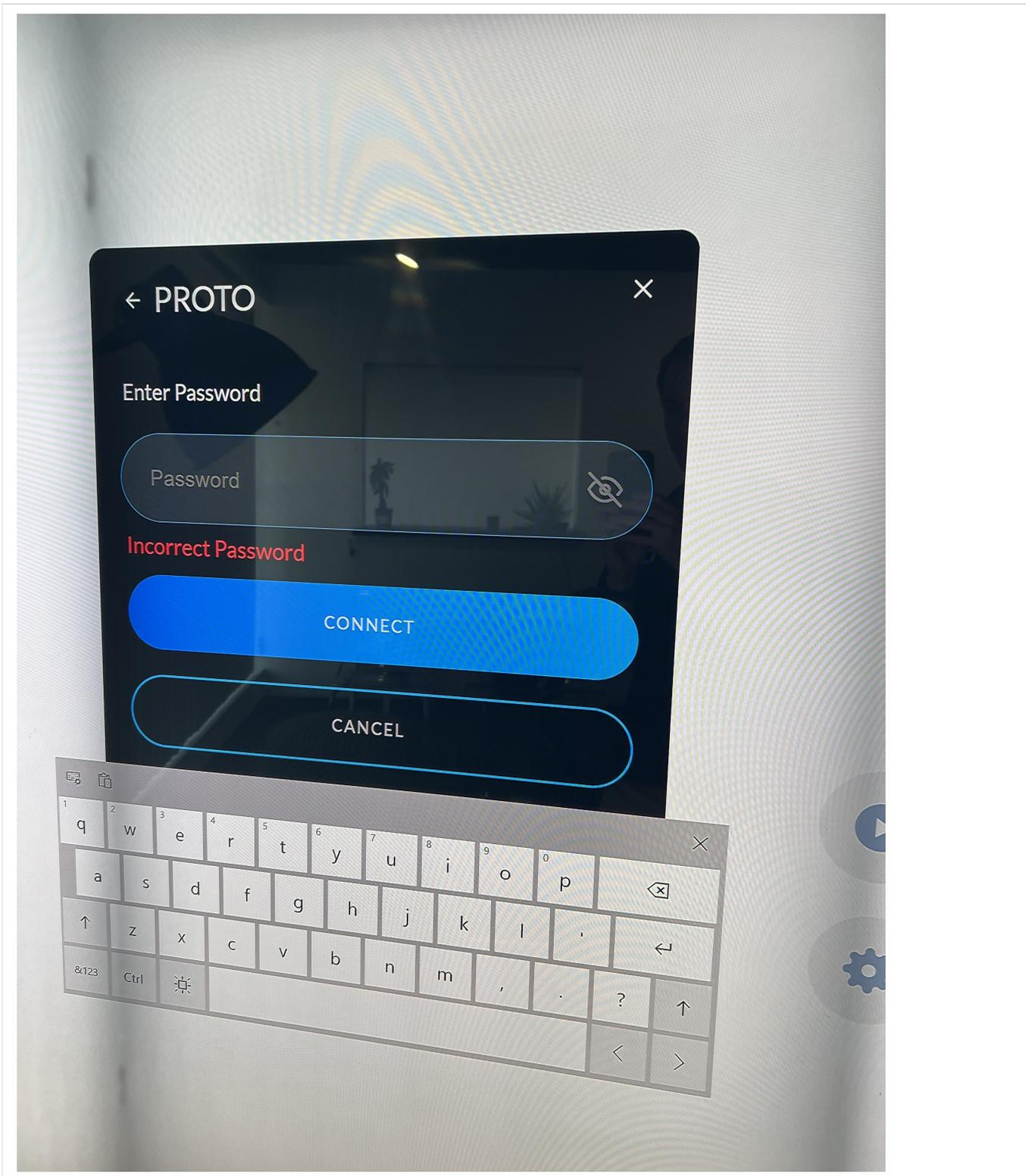
Once you've selected a network, you will be prompted to input a password, if any. Tap on the "Password" field to begin inputting a password. An on-screen keyboard will appear at the bottom of your Proto's touchscreen.
